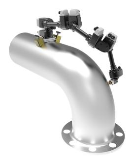
The R-Series Actuator is a full-featured robotic component as opposed to a simple servo motor. The output rotates continuously, requires no calibration or homing on boot-up, and contains a thru-bore for easy daisy-chaining of wiring. This enables the actuators to be used in everything from wheeled robots to collaborative robotic arms.
