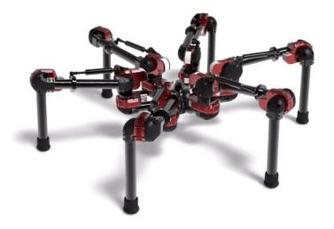
The X-Series Actuator<sup>®</sup> is designed to function as a full-featured robotic component as opposed to a simple servo motor. The output rotates continuously, requires no calibration or homing on boot-up, and contains a thru-bore for easy daisy-chaining and wiring. This enables these actuators to be used in everything from wheeled robots to multi degree of freedom collaborative robotic arms.
